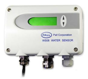
The Pall water sensor is option "W" on the Pall portable fluid purifier. This fast acting, highly repeatable in-line device measures relative humidity and temperature which are used to calculate parts per million (PPM) water content. Fluid relative humidity is the amount of dissolved water in a fluid expressed as a percentage of the amount of water necessary to cause 100% saturation. This in-line device provides instant feedback on water contamination of the fluid being purified.
